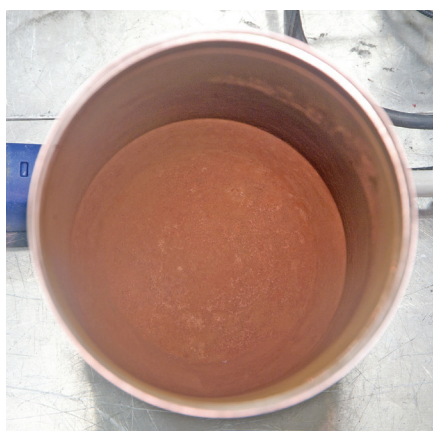
Figure 2. Corrosion observations at destructive examination (DE) of some 3013 containers packaged with hydrated \text{PuO}_2 /salt mixtures. Headspace and contact region corrosion was observed on the inner (left) and convenience (right) containers, respectively.
